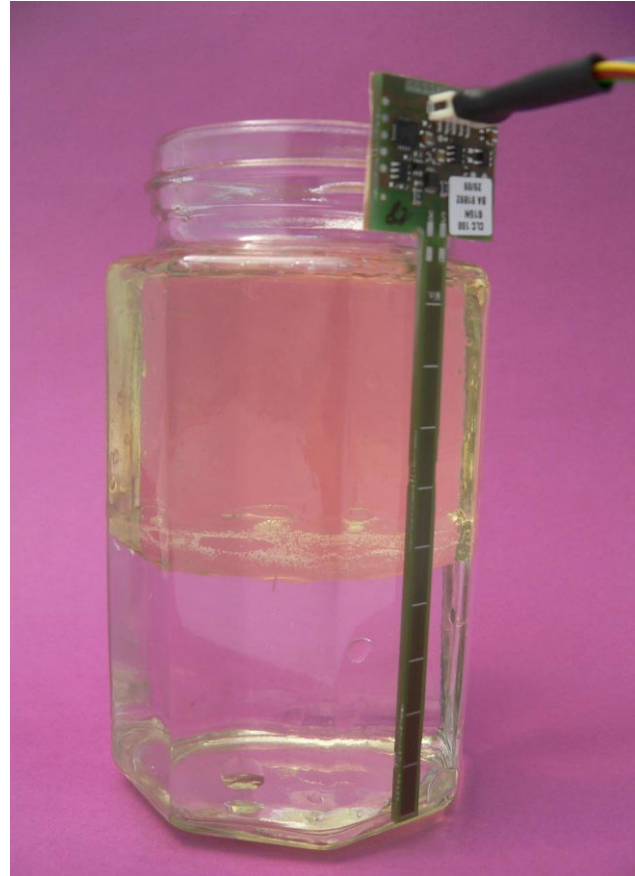
Fig. 1: Example of continuous oil over water detection with Sensortech's CLC sensor
